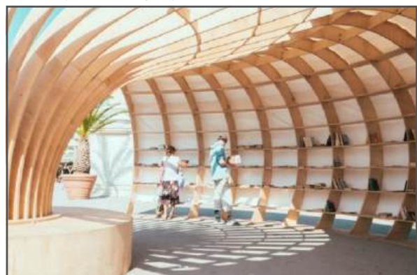
Fig. 3.6 A street library in Bulgaria that utilizes the tools of parametric design to create a wooden structure that is light and transportable (Photo by Emanuil Albert)
