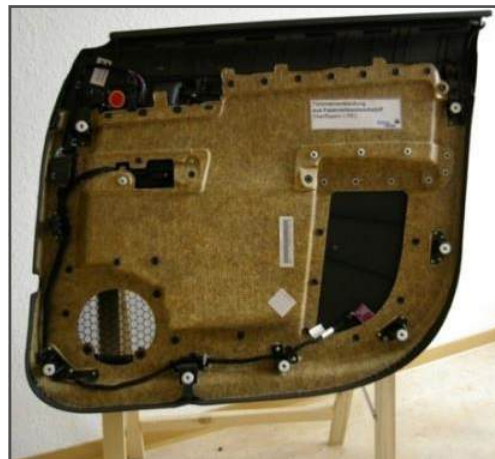
Fig. 7.1 Car panel made of hemp composite
