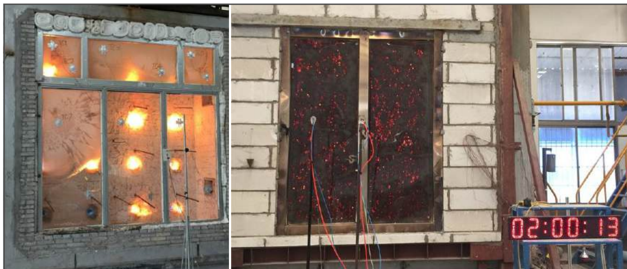
Fig. 3.16 Fire Doors under test (Source: http://www.firepros.hk/en/Service.aspx )
