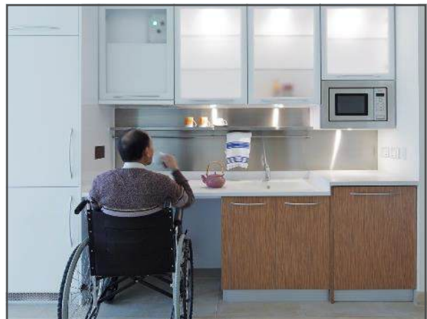
Fig. 4.60 Kitchen benchtops are lowered to 0.8m, and microwave cupboards are installed below 1.3m.
